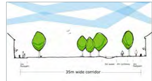
Section through Central Green Space
