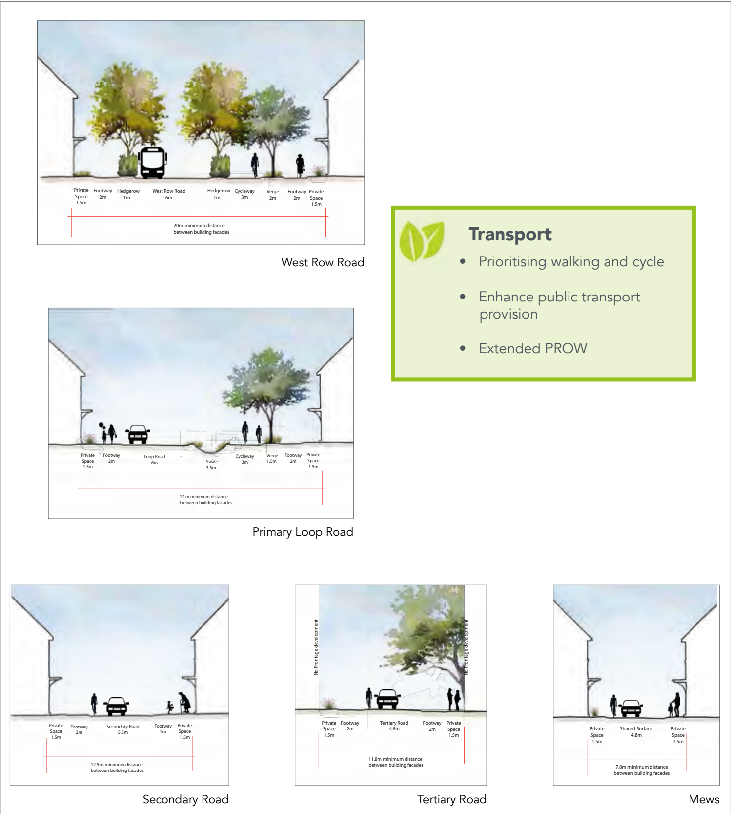
Figure 27 - Illustrative sections to show the minimum distances between buildings on different road types
